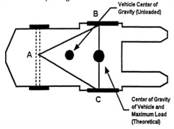
Notes: 1. When the vehicle is loaded, the combined center of gravity shifts toward line B-C. Theoretically, the maximum load will result in the center of gravity at line B-C. In actual practice, the combined center of gravity should never be at line B-C.
